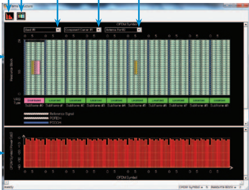
Frame Structure Screen (LTE-Advanced)
